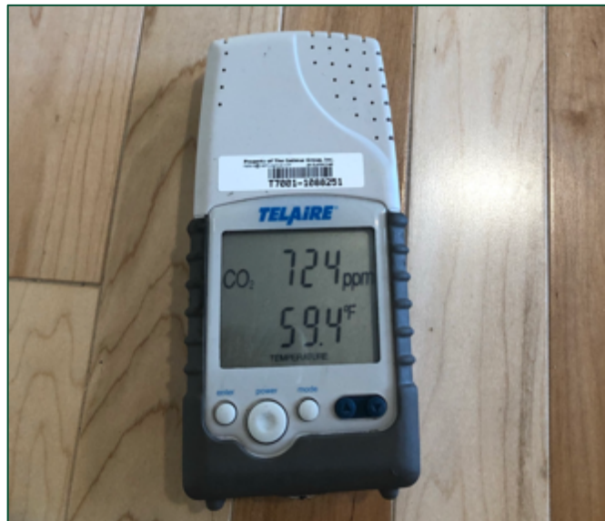
Figure 13. Interior CO 2 Reading
