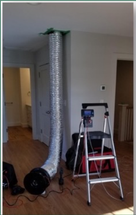
Figure 12. Duct Blaster® Attached to Ceiling Register
