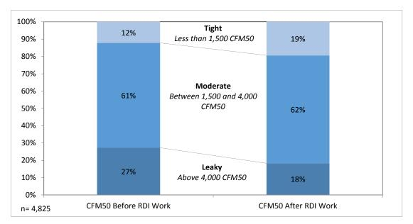
Figure 3-4. Leakiness of Homes, Before and After RDI Work
