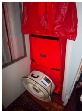
Figure 1. Illustration of Blower Door Testing
