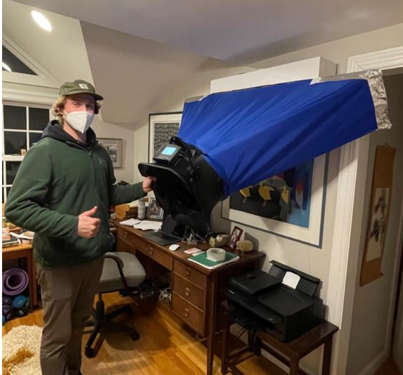
Figure 14. Technician Preparing to Collect Airflow Measurement
