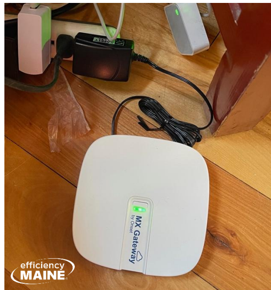
Figure 95. MX Gateway Uses Wi-Fi from Nano Router to Send Metered Data to Web
