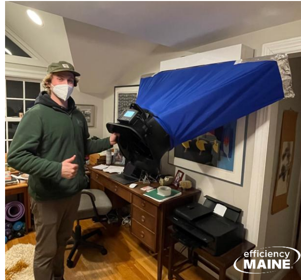
Figure 93. Technician Preparing to Collect Airflow Measurement Using Alnor Balometer
