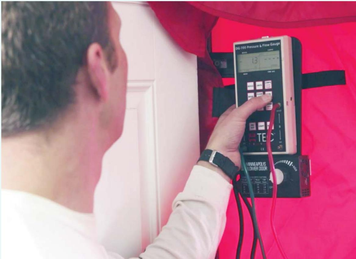
An energy audit can be a logical first step toward reducing energy waste. Energy advisors perform various tests to find the best ways to cut down on energy use in your home and suggest ways to take care of possible health and safety issues, including moisture, mold, and radon. Energy audits can include a walk-through of the entire home and tests using a blower door, combustion safety equipment, and a thermal camera.
